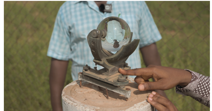
Inspecting faulty sunshine recorder at Yendi Meteorological Station (picture: James Merron 2024).
